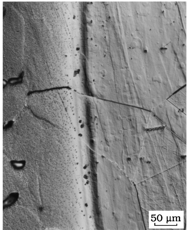
Figure 10 Optical micrograph showing the microstructural change across the Ni 3 Al-stainless steel interface.
